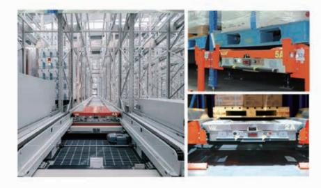
Radio shuttle racking system is a complete high-density storage system consisting of racks, shuttles and forklifts. This efficient storage method offers new options for increasing warehouse space utilization.
